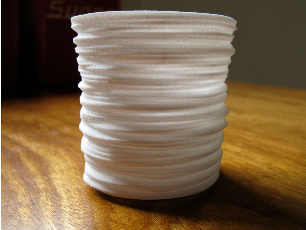
Figure 7: Measuring Cup - 3d print in laser sintered nylon
