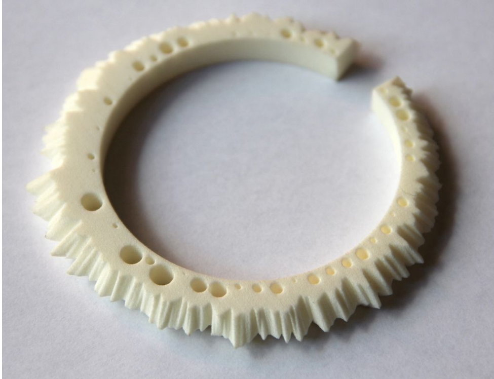
Figure 3: Weather Bracelet 3d printed in laser-sintered nylon
